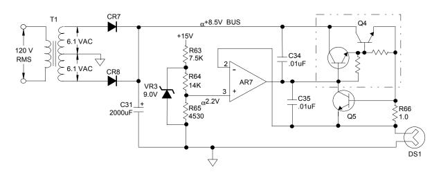
Figure 5-6. Detector Light Source Control Circuit
